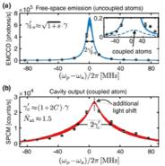
Fig. 1: Purcell broadening of a single rubidium atom in an optical fiber cavity. The upper panel shows the natural linewidth in free space, while the lower panel shows the broadening due to the coupling to the cavity.
