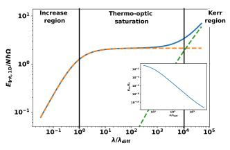
**Figure 4.** Interaction energy  $E_{\text{int,1D}}$  given by equation (37) for the experimental parameters  $N = 10^4$ ,  $\tilde{g}_K = 10^{-8}$ ,  $\tilde{g}_T = 10^{-4}$ , and  $\lambda_{\text{diff}} = 32$ . The orange dashed line shows the contribution of the thermo-optic effect, whereas the green dashed line indicates the contribution of the Kerr effect. The inset shows the interaction energy relative to the non-interacting energy  $E_0$  from (36).
