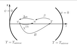
**Figure 1.** Sketch of the interaction mechanisms mediated by the dye solution. The change  $\Delta n$  of the refractive index n of the dye solution stems from both a Kerr nonlinearity  $\chi^{(3)}$  and thermo-optics described by the coefficient  $\beta$ . Reproduced from [22]. CC BY 4.0.
