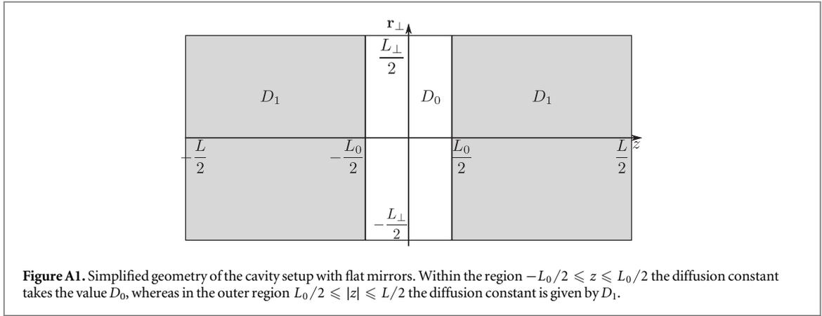
between the mirrors and of the mirrors themselves are denoted by  $D_0$  and  $D_1$ , respectively. Thus, the corresponding diffusion equation for the temperature difference  $\Delta T$  between the actual temperature of the experimental setup and the room temperature reads [49]
