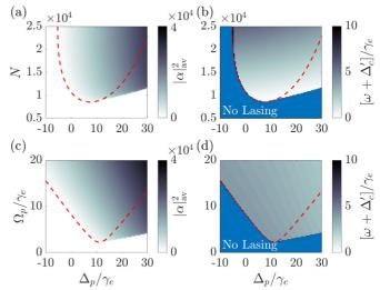
FIG. 4. Floquet method calculations of the intensity [(a) and (c)]and emission frequency [(b) and (d)] of the lasing field. The first row (a)–(b) show these values as a function of atom number and pump detuning while the second row (c)–(d) plots instead vary the pump Rabi frequency and pump detuning. The red dashed lines were calculated using Eq. (20). All parameters are the same as in Fig. 2.
