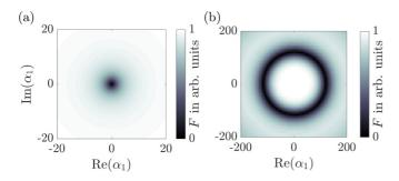
FIG. 3. (a) The function F defined in Eq. (30) in arbitrary units for N = 20000,  $\Delta_p = 10\gamma_e$ ,  $\Omega_p = 2\gamma_e$ ,  $\alpha_{-1} = 0$ ,  $\alpha_0 \approx -3.3 - 2.6i$ , and  $\omega > 0$ . (b) The function F for  $\Omega_p = 15\gamma_e$ ,  $\alpha_{-1} \approx 0$ ,  $\alpha_0 \approx -5.6 - 1.3i$ , and  $\omega \approx -205.5\gamma_e$ .
