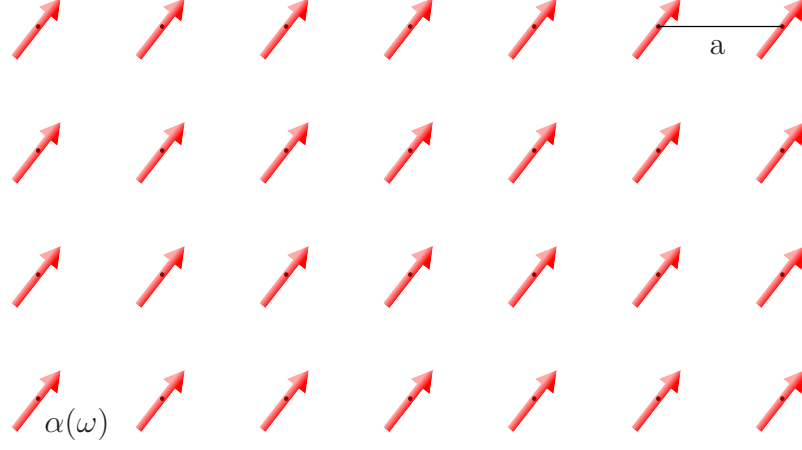
Figure 7.1: Microscopic model of a pure dielectric material. Polarizable particles with a polarizability \alpha(\omega) form a simple cubic lattice with lattice constant a .
