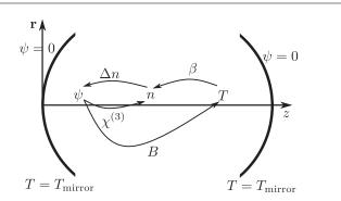
**Figure 1.** Sketch of the interaction mechanisms mediated by the dye solution. The change  $\Delta n$  of the refractive index n of the dye solution stems from both a Kerr nonlinearity  $\chi^{(3)}$  and thermo-optics described by the coefficient  $\beta$ . Reproduced from [22]. CC BY 4.0.
