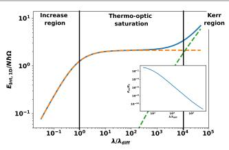
**Figure 4.** Interaction energy  $E_{\text{int,1D}}$  given by equation (37) for the experimental parameters  $N = 10^4$ ,  $\tilde{g}_K = 10^{-8}$ ,  $\tilde{g}_T = 10^{-4}$ , and  $\lambda_{\text{diff}} = 32$ . The orange dashed line shows the contribution of the thermo-optic effect, whereas the green dashed line indicates the contribution of the Kerr effect. The inset shows the interaction energy relative to the non-interacting energy  $E_0$  from (36).
