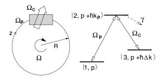
FIG. 1. (left) Setup of light Sagnac interferometer with vapor cell or trap attached to rotating body with angular velocity  $\Omega$ . (right) Level scheme of atoms. *p* denotes momentum along the peripheral direction *z*.  $k_p$  is the wave number of the probe field propagating parallel to *z*.  $\Delta k = k_p - k_c^{\parallel}$ , where  $k_c^{\parallel}$  is the component of the control-field wave vector in the *z* direction.
