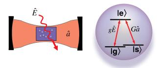
FIG. 1 (color online). Schematic diagram of the system: A quantized probe field  $\hat{E}$  interacts with an ensemble of  $\Lambda$ -type atoms driven by a cavity mode  $\hat{a}$  (left) in a Raman type coupling scheme (right).
