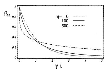
FIG. 6. Time dependence of excitation in spatially homogeneous, dense two-level medium. Time is in units of the inverse free-space decay rate.  $\eta \equiv N\lambda^2 d = 0$  (dotted), 100 (solid line), 500 (dashed line).  $g = \gamma / \sqrt{2 \pi \Delta_D} = 0.01$ .
