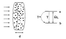
FIG. 9. Strongly driven, dense two-level medium.  $\gamma$  and  $\gamma^*$  describe radiative and nonradiative decays, respectively, and  $\Omega_L$  denotes Rabi frequency of local field.
