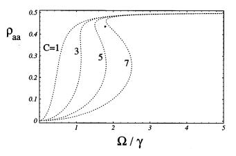
FIG. 10. Stationary excited-state population as function of driving-field Rabi-frequency  $\Omega$  for different cooperativity parameters. Here,  $\Gamma = \gamma^* = 0$ .
