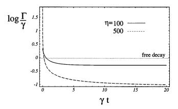
FIG. 7. Effective rate of decay  $\Gamma_{\text{eff}} = -\dot{\rho}_{aa}/\rho_{aa}$  for examples of Fig. 6. Dotted line corresponds to free-space decay. Amplified spontaneous emission in the initial phase and slowdown of decay in final phase are apparent.
