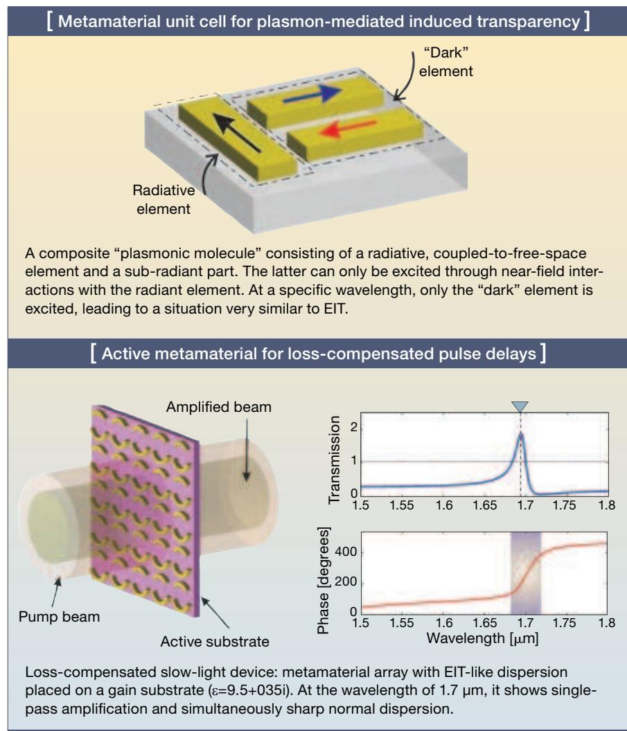
weakly coupled to free-space. Again, the latter element can be excited by the radiative element through electric or magnetic inductance, leading to a situation very similar to EIT. This analogy was unambiguously demonstrated by the same group very recently, by employing a variant of the meta-molecule suggested by X. Zhang.
